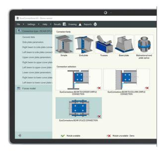
Design and verify the capacity of typical uniplanar frames & lattice connections in steel structures according to PN-EN 1993-1-8:2006 standard. Welded or bolted connections in various joints types.
